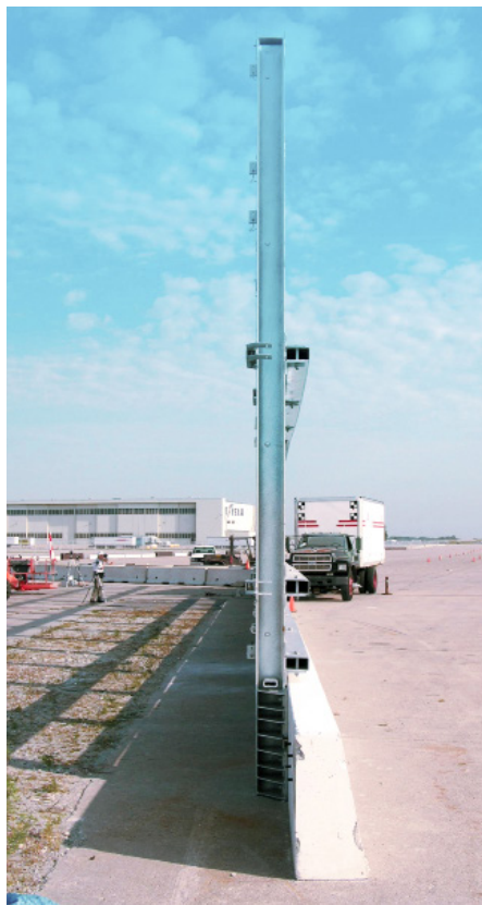
A 8,164kg truck impacts the TL-4 System at 60mph on a 25° angle
