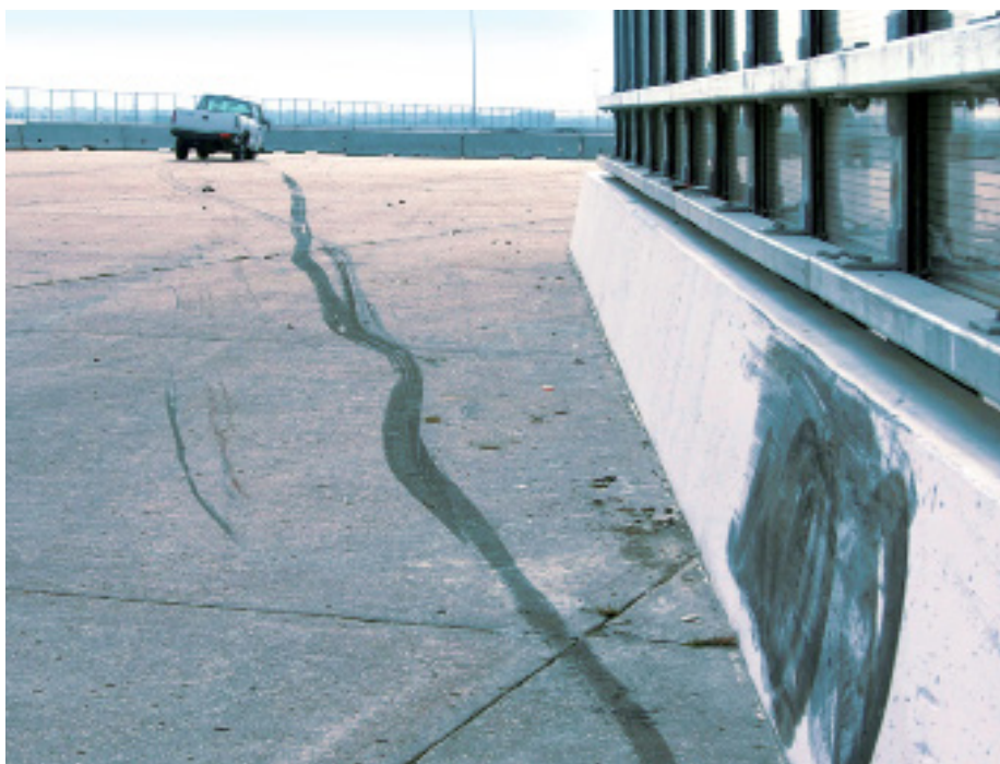
The soundstop TL-4 System stabilizes the vehicle after impact
