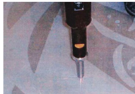
POINT 2 - CENTER IMPACT WITH CONCRETE TESTING HAMMER
