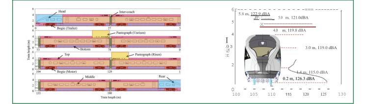
Tested at both high-speed and regular metro train speeds, the profile distribution of sound is similar across all trains. The speed at which it travels simply elevates the overall sound level (intensity/frequency).
