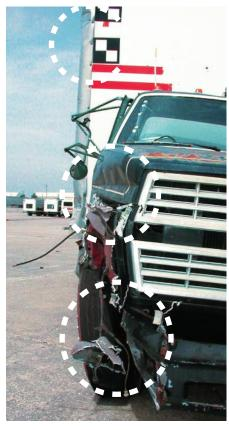
Damaged areas show how the TL-4 System reduces the severity of the crash
